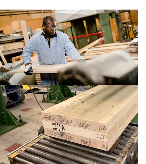
Michigan Tech plans to explore the possibility of mass timber as a main construction material for the Center for Convergence and Innovation. Mass timber consists of lumber glued together to form large structural elements. Michigan's forests are nearly 70 percent hardwoods, and mass timber construction provides a market for this important resource. Michigan Tech is a leader in the development of mass timber made from hardwood species in Michigan.
