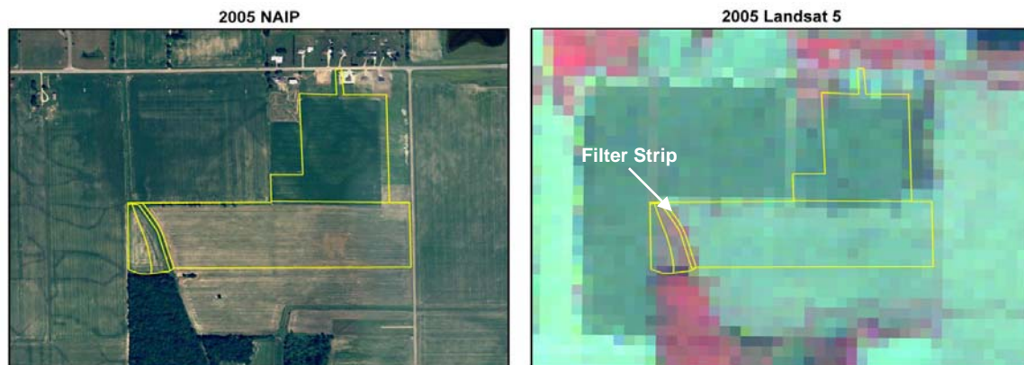
Figure 12: Filter Strip Implementation, Tract No. 13245, Clinton County Michigan; Landsat TM 5 (Bands 4, 3, 2). The filter strip is discernable in both the high-resolution NAIP image, and the Landsat image that can be used to map large multi-county areas.
