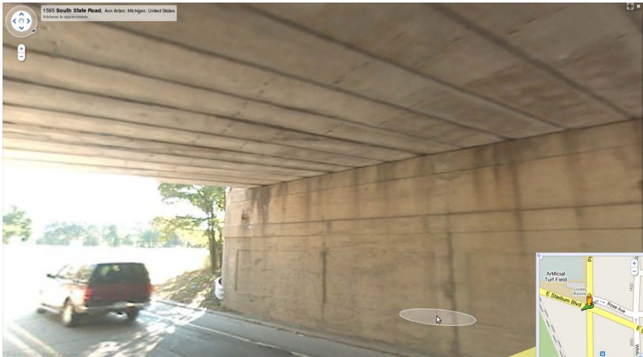
Figure 20: Example image from Google's StreetView showing the underside of a box-beam bridge in Michigan. With higher-resolution panoramas, such an interface could be extremely valuable to bridge inspectors and managers.
